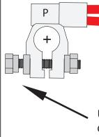
Unique battery connection bolt that allows for high draw accessories to be directly bolted to the battery.
