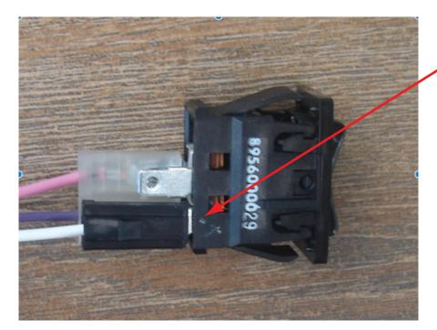
NOTE: Make sure you plug the connectors onto the rear wiper/washer switch as shown here)
