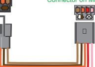
Plug these connectors onto your stock dash mounted 1990 rear wiper and washer switch.
