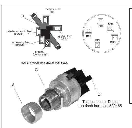
Completed ignition switch and dash mounting bracket assembly.
