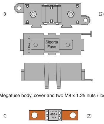
(Megafuse body, cover and two M8 x 1.25 nuts / lock washers)
