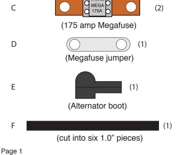
1. One this page, you will find the wire, fuse bodies, fuses, boot, ring terminals, and shrink tubing (items A through K) that are necessary to connect your alternator and main power feed for your new AAW wiring kit. Please be sure that all of the necessary components are present before starting this portion of your installation. If anything is missing, stop what you are doing and contact AAW at the number listed below right away.
