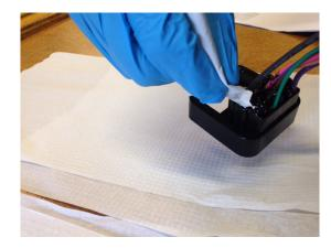
1. Place a sheet of paper towel or cardboard down to the area where you intend to work. Cut off the small applicator tip end of the grease packet, and apply the grease onto the connector as shown above.
