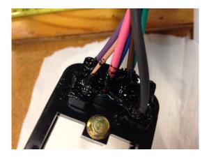
5. Your finished application should show no openings. Hold the connector up to light to see if there are any voids and touch them up. Apply a small amount of grease to the other side of the terminals to finish the job.
