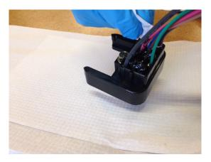
2. Apply grease until you have covered all of the ends of each of the terminals and cavities.
