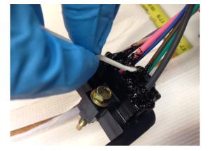
4. After working the grease into the cavities, begin smoothing it out to give it a cleaner, more finished appearance. If you need to apply additional grease, that is OK.
