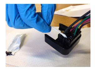
3. Once you have completed applying the grease, set the tube down onto your working surface. Use the cotton tipped applicator stick to work the grease into the cavities.
