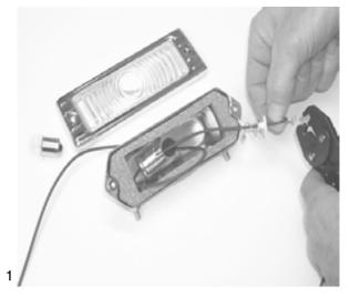
Photo 1 shows the spring R and wafer P installed onto the brown wire prior to rivet Q being crimped onto the brown wire.
