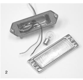
Photo 2 shows the same method as photo 1, but applies to a dual wire parking lamp (brown and blue wires). You must re-use your orignal 2 hole wafer insert over as it is NOT included in this kit.
