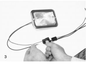
Photo 3 shows the finishing of a parking lamp pigtail assembly using terminals N and connector L. The pigtails will connect to the 500432 front light harness using terminals H or J along with connector M as shown on page 7 of this instruction set.
