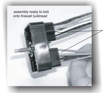
apply silicone sealant to back side of connector after installing terminals
