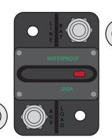
NOTE: This circuit breaker should be mounted as close to the battery power source (junction block, starter relay, starter solenoid, etc.) as possible. AAW does NOT recommend installing this kit inside of the vehicle as the main powerfeed from the battery source to the circuit breaker is an unfused lead, and as such, should not be routed to the inside of your vehicle.
