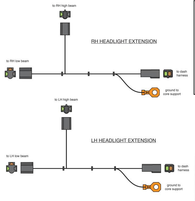
NOTE: In this kit, you will find the left hand and right hand Headlight Extension Harnesses. They are completely assembled and require no additional work other than plugging them onto the dash/main harness, P/N's 510392 (1966-67 Fairlane and Comet), or 510554 (1962-65 Fairlane & 1962-63 Mercury Meteor) and the Low and High Beam Headlight Bulbs (see specific instructions on P/N 510391 or P/N 510553, pages 12, Figures A).
