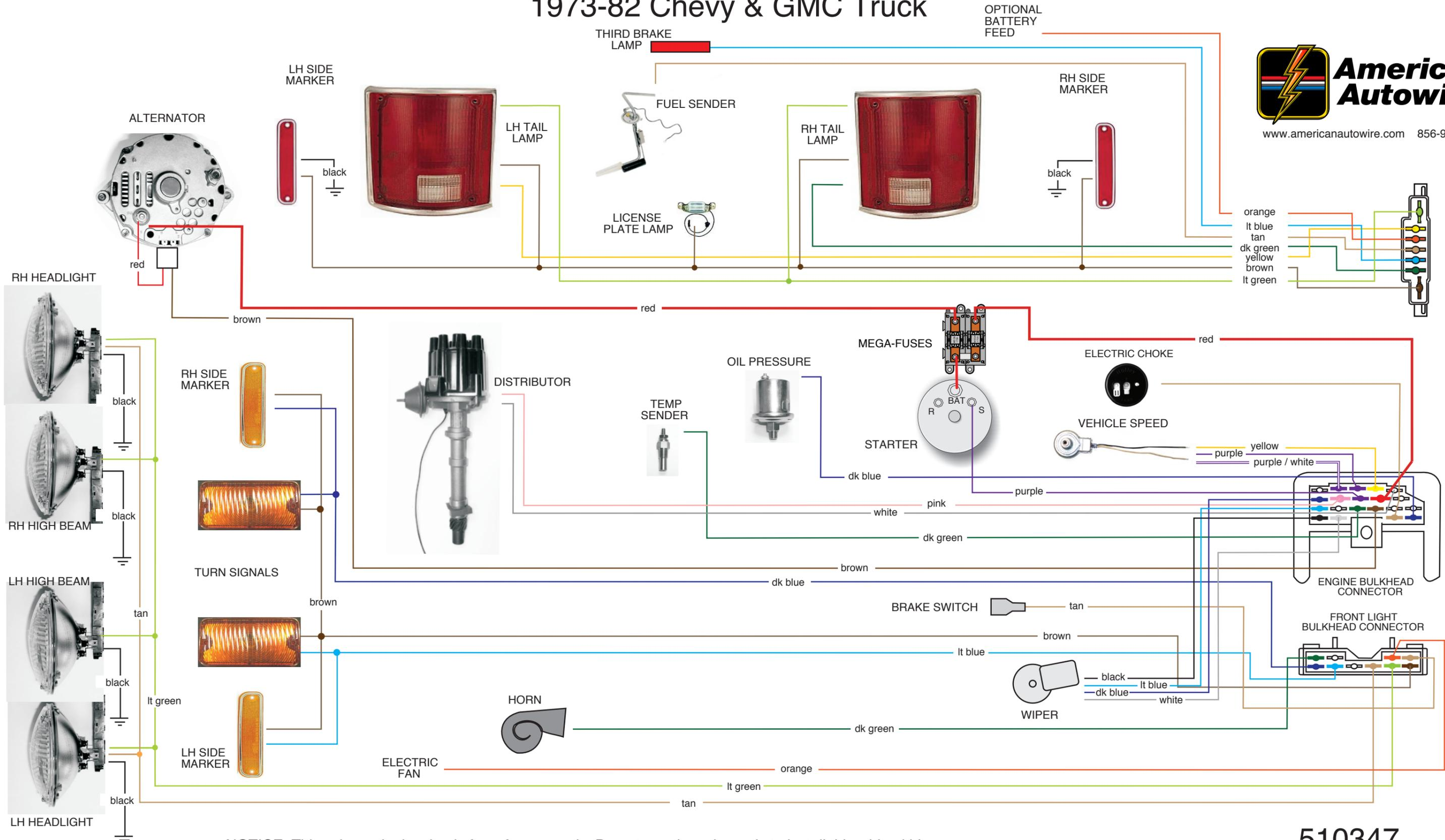
**NOTICE:** This schematic drawing is for reference only. Do not use the schematic to install this wiring kit! Use the instruction sheets included in each bag, which includes directions for proper terminations, and specific applications).
