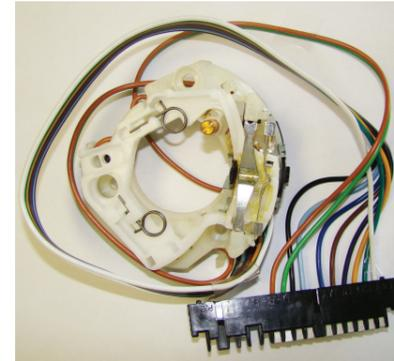
OEM steering column turn signal switch.
