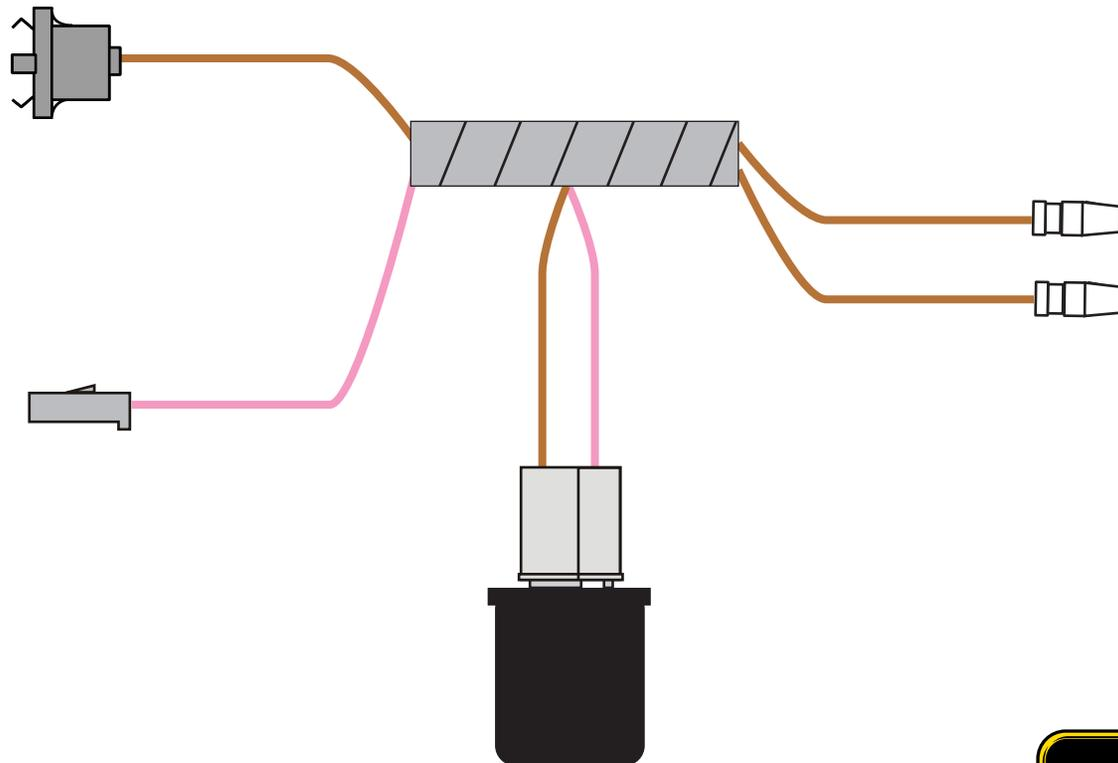
Plug these 2 leads into your stock original parking brake warning lamp switch assembly.
