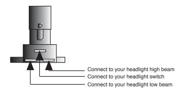
Connect the Dimmer Switch wires as shown above.
