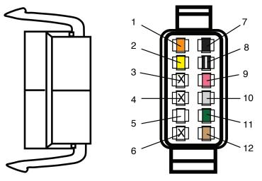
**GAUGE HARNESS CONNECTOR** SUPPLIED ON THE CONSOLE EXTENSION HARNESS (viewed from the terminal side opposite of the wire entry)
