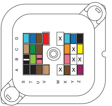
1968 - 1969 FUSE BLOCK BULKHEAD CONNECTOR
