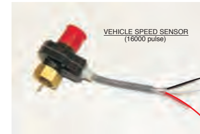
Typical 3 wire Autometer 5291 VSS connection
