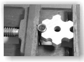
**STEP 2:** Set the crimp tool in a vise, as shown, with the terminal set into position.
