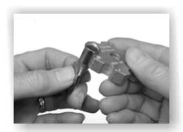
STEP 1: Select the proper gauge location which matches your cable. Orient the terminal, as shown above.
