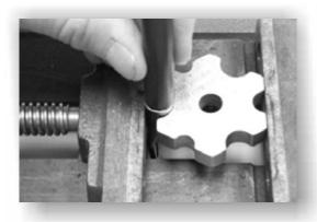
STEP 5: Seat the cable as far into the terminal as it will allow. Tighten the vise as far as you can, to apply proper crimp on the terminal.
