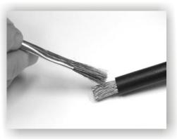
STEP 3: Strip the cable to 5/8", and apply rosin solder flux. A protective sleeve (shrink tube) should be slid onto the cable at this point if you are using one.
