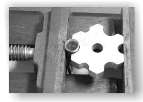
STEP 2: Set the crimp tool in a vise, as shown, with the terminal set into position.
