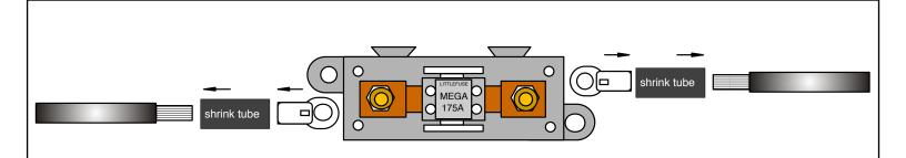
NOTE: This Mega-Fuse box should be mounted as close to the battery power source (junction block, starter relay, starter solenoid, etc.) as possible. AAW does NOT recommend installing this kit inside of the vehicle as the main power feed from the battery source to the Mega-Fuse is an unfused lead, and as such, should not be routed to the inside of your vehicle.
