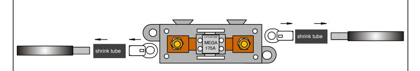
NOTE: This Mega-Fuse box should be mounted as close to the battery power source (junction block, starter relay, starter solenoid, etc.) as possible. AAW does NOT recommend installing this kit inside of the vehicle as the main power feed from the battery source to the Mega-Fuse is an unfused lead, and as such, should not be routed to the inside of your vehicle.
