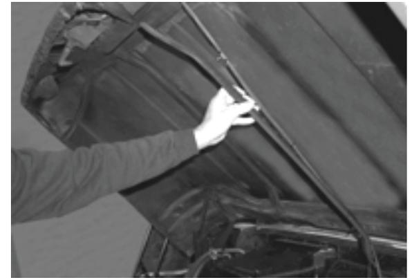
Route wires along hood support, and attached with the supplied clips. Be sure to protect wires along any sharp edges. Re-install hood support.
