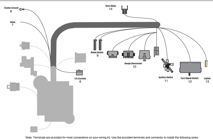
Note: Terminals are provided for most connections on your wiring kit. Use the provided terminals and connector to install the following wires:
