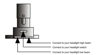
Connect the Dimmer Switch wires as shown above.
