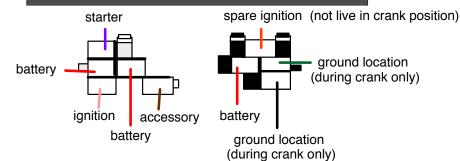
connection to the: Highway 22 wiring system Power Plus 13, 16, and 20 wiring systems
