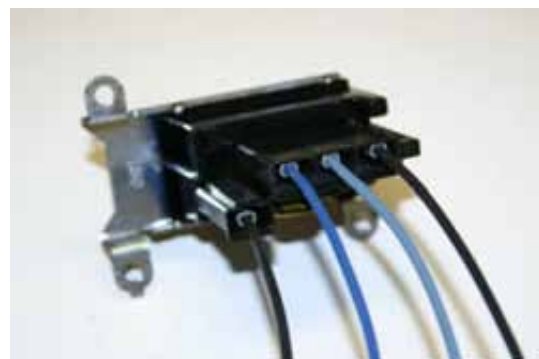
The above picture shows the orientation for 1972 Nova wiper hook-up only . All other applications can only be plugged in one way.
