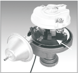
p/n 38131 Breakerless Ignition Module, GM V-8 POINT CONVERSION KIT
