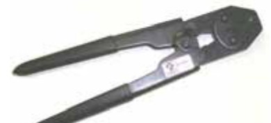
p/n 500649 Multi-crimp tool (20-14 gauge).
