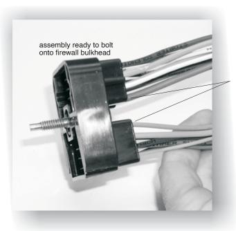
apply silicone sealant to back side of connector after installing terminals
