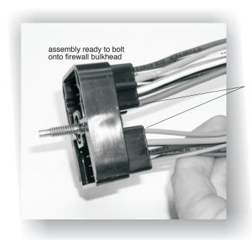
apply silicone sealant to back side of connector after installing terminals
