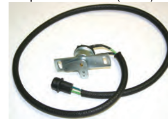
Muncie 4 speed back up lamp switch. p/n 01993307 (1966-67) p/n 01993431 (1968)
