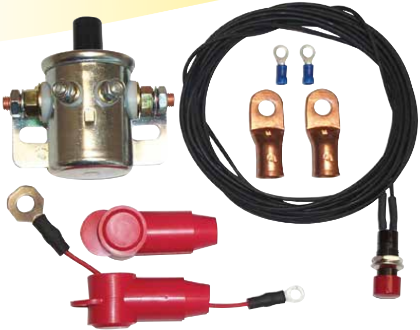
500834 Remote Master Disconnect Switch Control your battery disconnect with a small remote mounted switch. Can be used with remote control modules. SPST latching solenoid with two 5/16" studs. Rated at 110 amp continuous. ..... 120.00 ea
