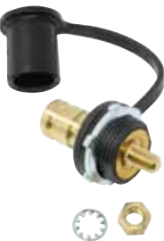
500011 Battery Jumper Stud Negative, with insulated cover. 3/8"-16 threaded brass stud mount. 13/16" dia x 1-1/8" long. Requires 1-9/32" hole. ..... 20.00 ea
