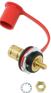
500010 Battery Jumper Stud Positive, with insulated cover. 3/8"-16 threaded brass stud mount. 13/16" dia x 1-1/8" long. Requires 1-9/32" hole. ..... 22.00 ea
