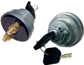
500713 Secure Keyed 2 Pole Battery Disconnect 2-3/8" battery studs, indexing posts with security feature. 3/4"-16 thread, fits 3/4" hole. 6 to 36 volt. 180 amp continuous and 1000 amp surge. ..... 40.00 ea
